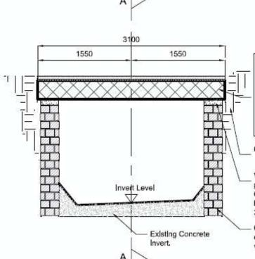
Proposed prefabricated reindorced concrete slab by Shay Murtagh OSA. Prefabricated slabs to withstand typical live loading to maximum of 40 tonnes + 30HB Units and to be designed with current British design standards and regulations. Environmental factor to be considered - Burled, Wet rarely dry, freeze / thaw & de-icing salts, Contractor is to make allowance within his design for waterproofing system to be in accordance with appropriate standards.
